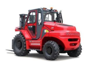
GOODSENSE 3 TON 4 WHEEL DRIVE ROUGH TERRAIN FORKLIFT IS A 4×4 MODEL FOR INDUSTRIAL USE. IT LIFTS 3,000 KILOS TO A HEIGHT OF 4.35 METRES. IT IS FITTED WITH A FOUR CYLINDER HATZ ENGINE THAT PRODUCES 54.9KW AND A TOP SPEED OF 25KM/H WHEN THE FORKLIFT IS EMPTY LOADED.
