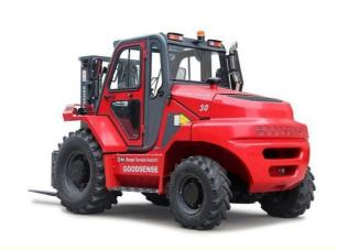
GOODSENSE 3 TON 4 WHEEL DRIVE ROUGH TERRAIN FORKLIFT IS A  $4\times4$  MODEL FOR INDUSTRIAL USE. IT LIFTS 3,000 KILOS TO A HEIGHT OF 4.35 METRES. IT IS FITTED WITH A FOUR CYLINDER HATZ ENGINE THAT PRODUCES 54.9KW AND A TOP SPEED OF 25KM/H WHEN THE FORKLIFT IS EMPTY LOADED.
